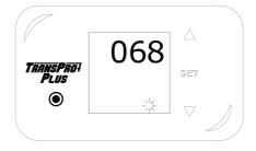
**11.3** Press "set" button to select "ctr" mode, press up and down button to set value at 0 or 1, 0 for celsius, 1 for Fahrenheit
