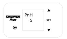
**14.5** For "PnH" value, if customer set value with "0", then in the main screen of control board there is no pre-setting indicator shows at the bottom left corner.
