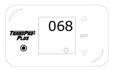
**12.3** Press "set" button to select "Pb" mode. Press up and down button to make temperature calibration.
