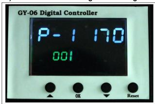
When there is temperature difference between SV (current heating temperature shows on the display screen) and actual Temp of heat platen, please long press button for 5 seconds to enter the PI1 mode to calibrate.
