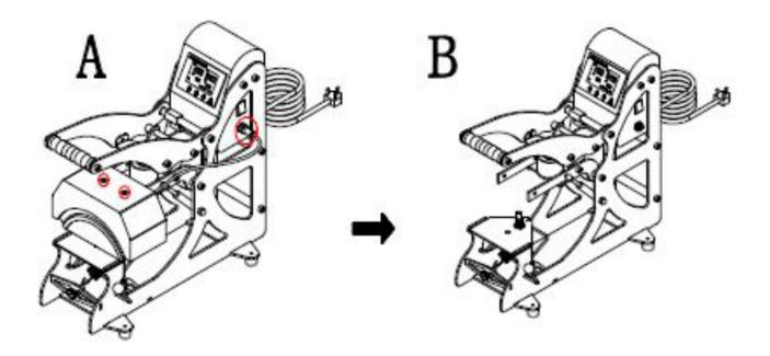
Remove the male socket which is connected to Female socket set in side of electrical case; Unscrew two screws on the cap heat platen.
